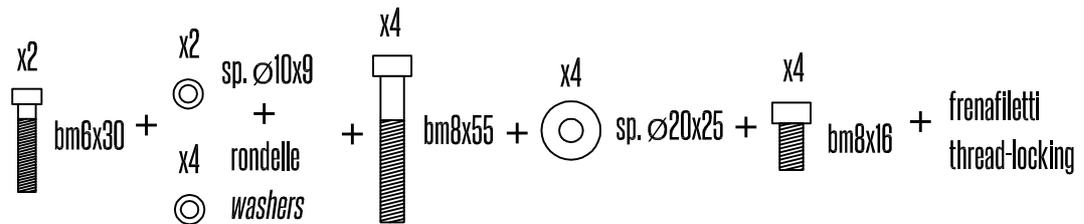
x2 bm6x30 + x2 sp. Ø10x9 + x4 rondelle washers + x4 bm8x55 + x4 sp. Ø20x25 + x4 bm8x16 + frenafilotti thread-locking
